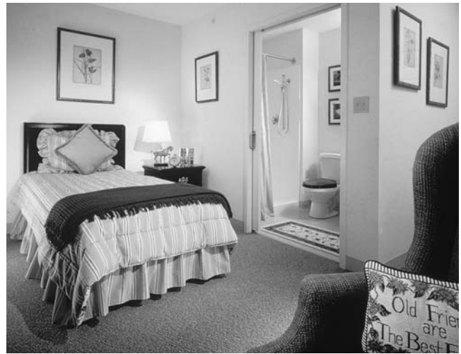
Toilet is visible from the resident's bed: In the Goddard House (page 169), a wide pocket door has been situated so that a view into the bathroom is possible. (Photo: Edward Jacoby Photography)
